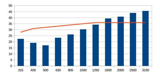
The spectrum of acoustic insulation of the cabin in third octave bands.
