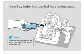
Set the chair upright after inserting the center groove of the base into the cylinder.
