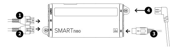
**NOTE** All cables must be connected to the control box in this specific sequence before you plug in the power.
